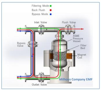
upset the bed and tumble the balls which knock the corrosion products from their surfaces. This tumbling occurs within 15 seconds and is largely responsible for the tremendous bed-life of the matrix which will last for approximately 40 years.
